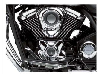
Both pistons are connected to a single crank pin.
