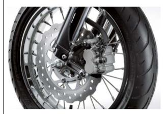
Petal brake discs front and rear provide superb stopping power. In addition to helping reduce unsprung weight, the wave shape of the petal discs helps clean the brake pads for more efficient braking performance.
