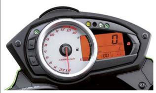
Analogue-style tachometer is complemented by an LCD display with digital speedometer, odometer, tripmeter, water temp, fuel gauge and clock.
