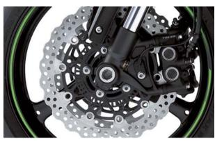
Dual brake pads (instead of 4 individual pads) are used in the Tokico radial mount calipers.
