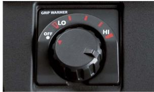
The temperature control switch is located on the left fairing for easy access.
