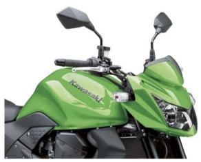
Aggressive bikini front cowl with twin-bulb, multireflector headlight.
