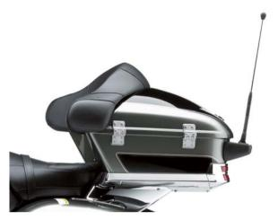
The 50 litre lockable trunk is large enough to fit two full-face helmets.
