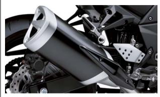
Short-style silencer features an exhaust device added just upstream of the silencer entrance to help "tune" back pressure waves for enhanced response in the low-mid range.
