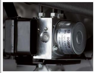
KIBS uses the world's smallest and lightest ABS unit and is also the first mass produced motorcycle system where the engine ECU communicates with the ABS system.
