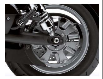
Belt drive is quieter and requires less maintenance than a chain and is lighter than a shaft drive.
