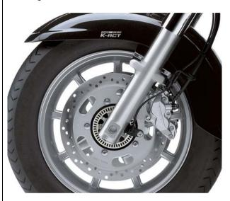
The coactive function is disengaged at speeds below 20 km/h (12 mph) for maximum control in tight turns and the ABS function is disengaged below 6 km/h (4 mph).
