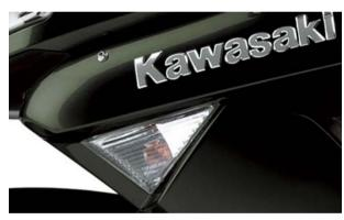
■ The front turn signals are integrated into the front cowl, while the rear signals are easily visible, even with panniers.
