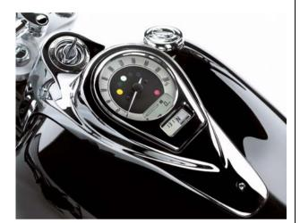
Multi-function LCD displays on the tank mounted instrument cluster are controlled by switches on the right handlebar. Features include a gear position indicator, fuel gauge, clock, odometer, dual trip meters, remaining range and average fuel consumption.
