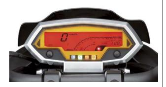
The fully digital instrument panel includes digital speedometer, bar-style digital tachometer, odometer, two trip meters, fuel gauge, and clock.
