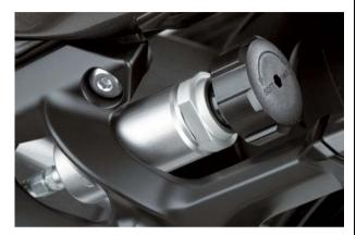
The rear suspension has adjustable rebound damping, and preload can be adjusted via a remote hydraulic adjuster.
