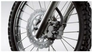
Petal brake discs front and rear provide superb stopping power. In addition to helping reduce unsprung weight, the wave shape of the petal discs helps clean the brake pads for more efficient braking performance.
