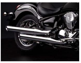
Honeycomb type catalysers are located in the mufflers and help the VN900 meet stringent EURO-III regulations.
