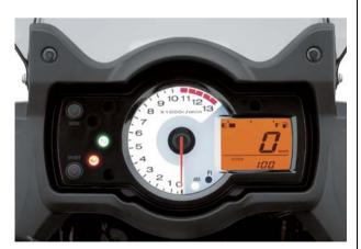
The instrument panel features white LED backlighting for increased visibility at night. Features include a digital speedometer, analogue-style tachometer, digital fuel gauge, odometer, dual trip meter, clock and LED indicator lamps.
