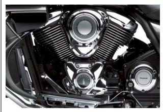
Large capacity air boxes are located on either side of the engine.
