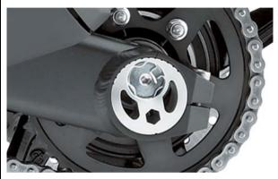
The swingarm features eccentric axle adjusters for easy adjustment.
