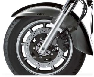
The coactive function is disengaged at speeds below 20 km/h (12 mph) for maximum control in tight turns and the ABS function is disengaged below 6 km/h (4 mph).
