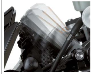
■ The meter can be easily repositioned using the adjuster on the left side.
