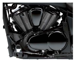
■ The finned cylinders and heads combine with liquid cooling to provide exceptional thermal control.
