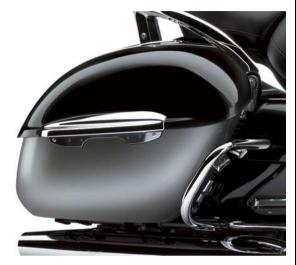
Top opening panniers are sealed and lockable, with a volume of 38 litres each.
