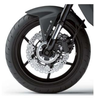
■ The ZR750M model is fitted with an ABS system to prevent wheel lock up during heavy braking.
